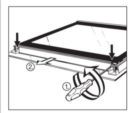
■ Unscrew the Torx screws, and remove the guides, trim and seal.
